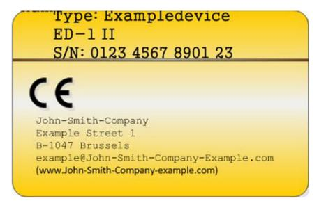
Template of a correct data plate for an importer (instead of a name a registered trade mark could also be used):
